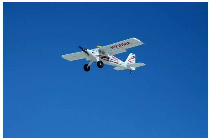
James Baer's Timber carrying a camera above the wing shown flying nearly stationary in the head wind with partial flaps deployed.
